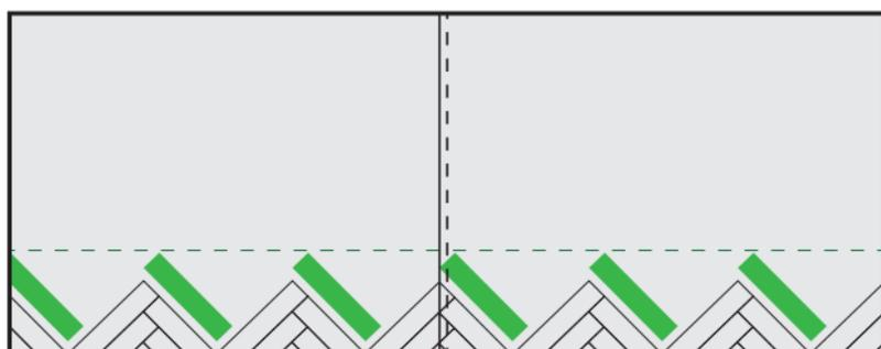
Now install B-planks and cut the most right piece to size.
