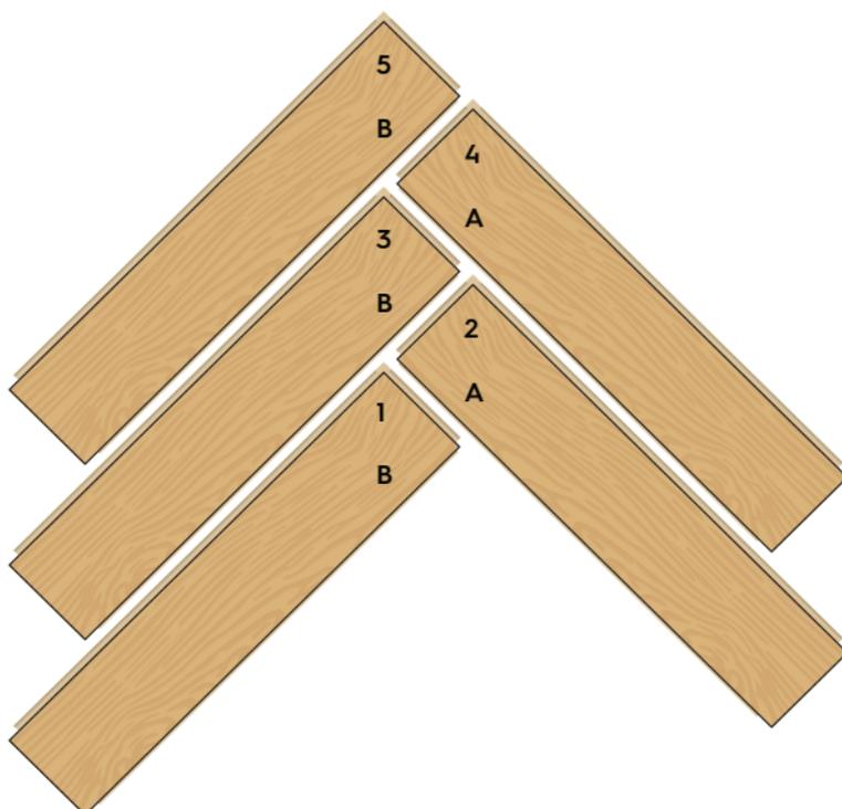
Install the boards precisely and in the order indicated by the numbers on the boards. Carefully check the joints between the planks after every plank which is added. No protruding edge may be felt!
