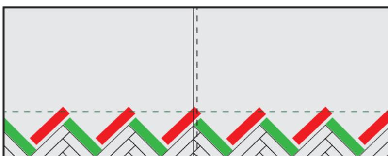
This alternating installation of A-planks and B-planks continues throughout the whole room. It is important to check frequently that:
